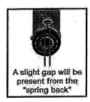
5. The locator will "pop off" after the second clamp is crimped and can be discarded. The result is a clean appearance and a reliable assembly.
