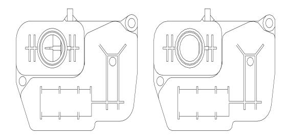
5.4 Have a helper slowly rotate the temperature dial from full cool (blue), to full heat (red) while you are watching the white valve gate. As the dial is rotated towards full heat, gate movement should be seen. A small slot will slowly appear, and then a larger opening will appear as the valve fully opens. Then have the helper slowly rotate the temperature dial back to full cool (blue). The valve gate should now move slowly to the closed position.
