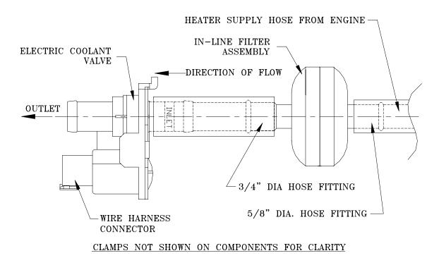
Place a clamping device on the inlet side of the reducer fitting that connects the 5/8" supply hose to the 3/4" hose on the inlet side of the valve (clamp on 5/8" hose). Place a second clamping device between the coolant valve and base unit (clamp 3/4" hose on outlet side of valve). Remove the reducer fitting, capturing the coolant in a pan. Remove the short section of 3/4" hose attached to the inlet side of the valve.
